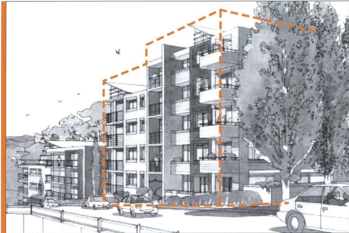
01.50. A building envelope is not a building. It defines a generous three-dimensional space within which quality residential design can occur.
